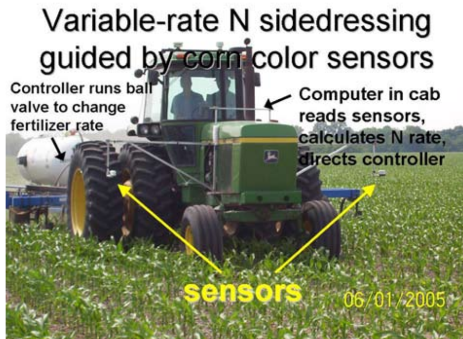
Figure 1. Crop sensors can diagnose corn N need based on color and control variable-rate sidedressing to accurately meet crop needs. Demonstration fields in 2009 have (so far) been highly variable in crop
